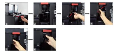
**Step 2:** Remove the cover of the mixer device, remove the mixing bowl and clean it with water.
