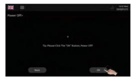
Step 4: In Power Off Mode, open the door with the key, press the power button and then lock the door.
